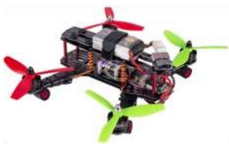
Drone with camera and US sensor
