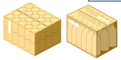
Smart labels should be attached on positions where you can find a sufficient distance to the content of a packaging.
